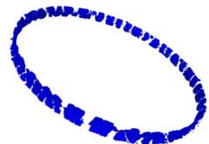
Fragmenting steel cylinder using stochastic material properties
